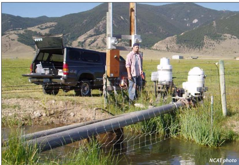
Use only the oil recommended by the manufacturer. Tag each engine with a label identifying the proper oil.
