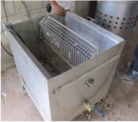
A typical scalding tank that can handle four to six birds at a time. Photo: NCAT
