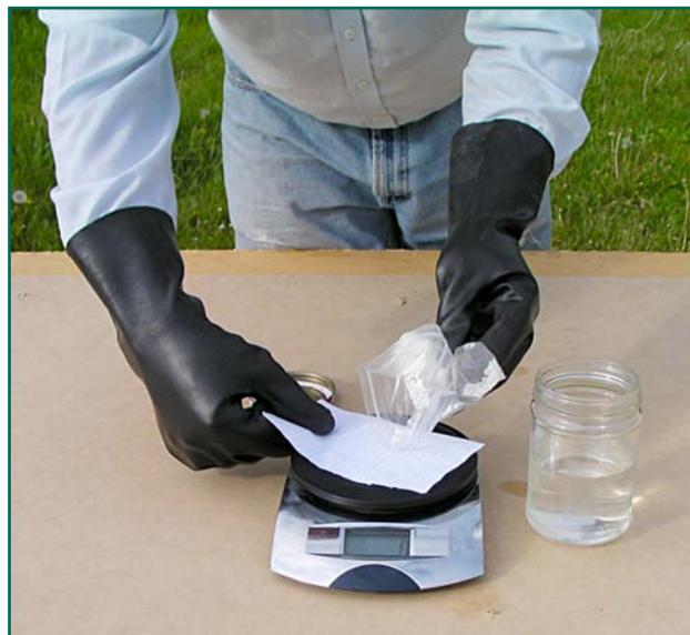
Measure 4 grams of sodium hydroxide or 5.6 grams of potassium hydroxide using your scale. Add the catalyst to your clean glass mixing jar.
