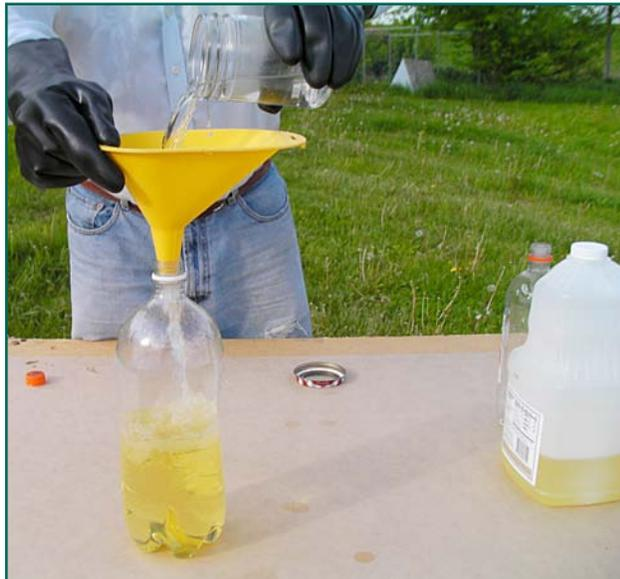
Add the methoxide solution to your oil. Use a funnel and be careful not to spill. If you spill, clean up the material immediately with paper towels and dispose of the contaminated paper towels safely.
