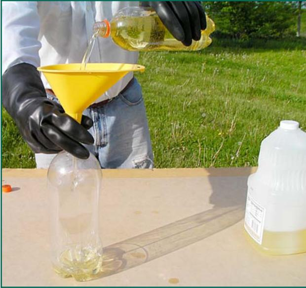
Measure 1 liter of oil, and use your funnel to pour it into the 2-liter soda bottle. You will get a better reaction if the oil is warm. About 140 degrees Fahrenheit is ideal. You can heat the oil in a pan on the stove or just leave it in the sun for an hour. If you choose to pre-heat the oil, be very careful not to get the oil hotter than 140 degrees.
