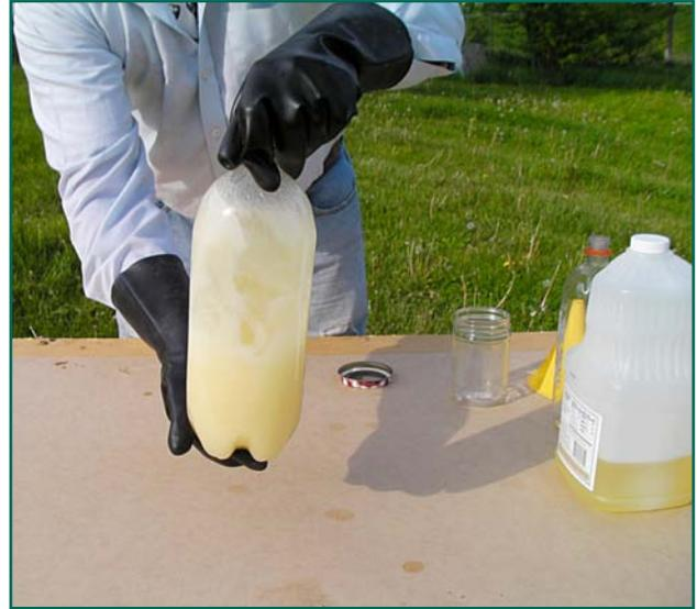
Allow the bottle to stand for an hour. The mixture will begin to clear almost immediately and a layer of darker liquid will begin to form on the bottom of the bottle.
