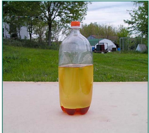
You can now drain off the glycerol by taking off the bottle cap, covering the open mouth of the bottle with your thumb, and inverting the bottle. Wear gloves. Allow the glycerol to collect in the neck of the bottle and then use your thumb as a valve to drain the darker liquid into another container. Discard the glycerol by composting or use it as a degreaser. What remains in the bottle is useable biodiesel.
