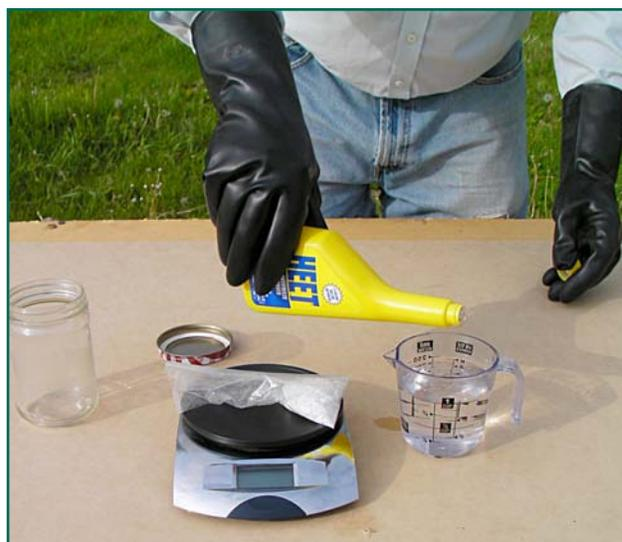
Measure 250 milliliters of methanol, using a graduated beaker or measuring cup. Add the methanol to the glass mixing jar with the catalyst.
