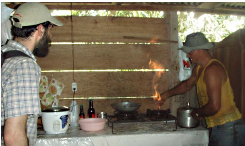
A farmer in Costa Rica exhibits the amount of gas available from his digester. Photo by Ian Woofenden.
