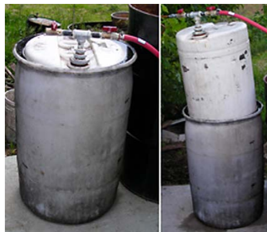
A simple floating-top digester built from scrap materials. Photo by Rich Dana.
