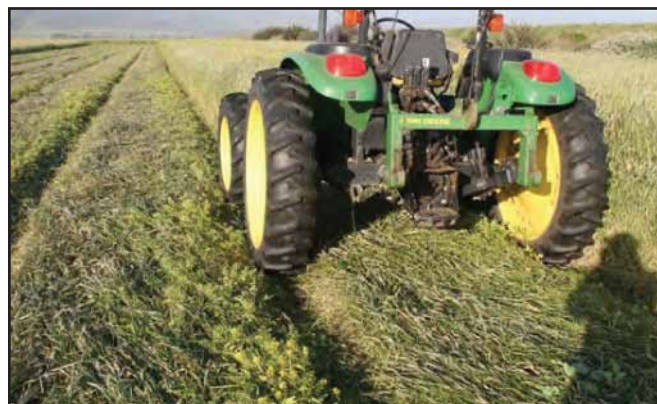
Figure 17: Terminating cover crops on beds using a roller crimper. (Eric Brennan)
