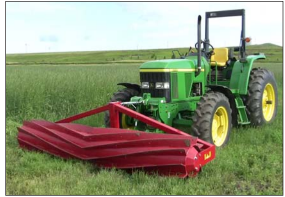
Using a roller-crimper to terminate a cover crop of cereal rye in Dickinson, North Dakota. Learn more about roller-crimpers and no-till grain production by viewing ATTRA's free online webinar, Innovative No-Till: Using Multi-Species Cover Crops to Improve Soil Health , www.attra.ncat.org/video/#notill Photo: Susan Tallman, NCAT
