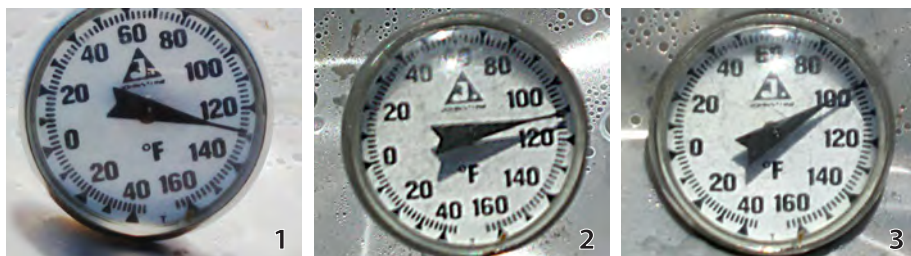
Surface temperature (1), temperature at three inches deep (2), and temperature at six inches deep (3). Photos: Martin Guerena, NCAT
