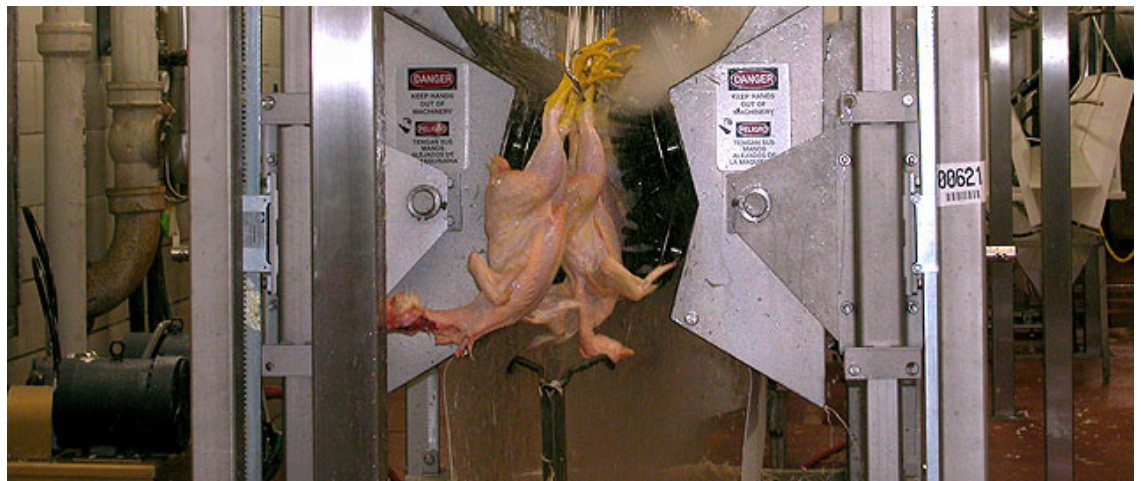
Broiler carcasses exiting an automated feather-picking machine. Photo: Mark Freeman
