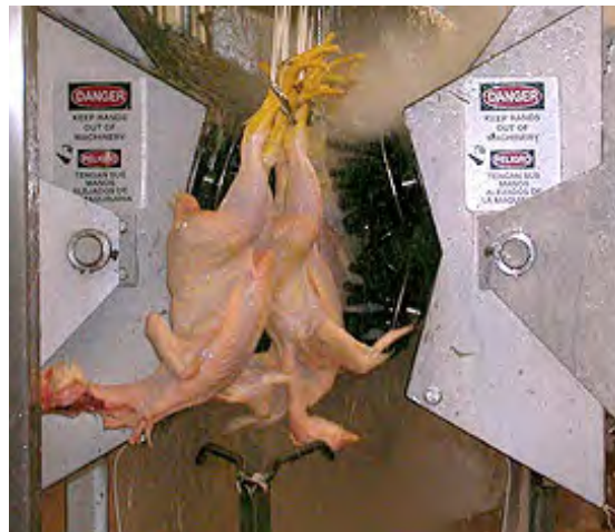
Broiler carcasses exiting an automated feather-picking machine. Photo: Mark Freeman
