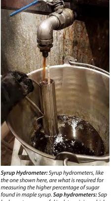
measuring the higher percentage of sugar found in maple syrup. **Sap hydrometers:** Sap hydrometers are useful in determining which trees have sweeter sap and for calculating how many gallons of sap it will take to make one gallon of syrup according to Jones Rule of 86. Photo: Josh Penick, Hijinks Farm (NH)
