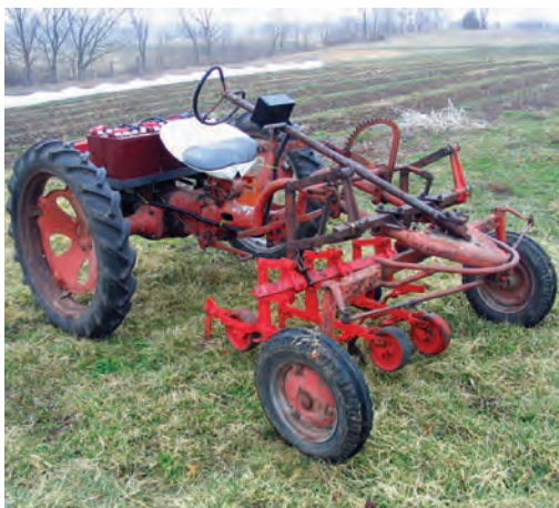
An Allis Chalmers G converted to electric at Fair Share Farm, Kearney, Missouri. Photo: Rex Dufour, NCAT
