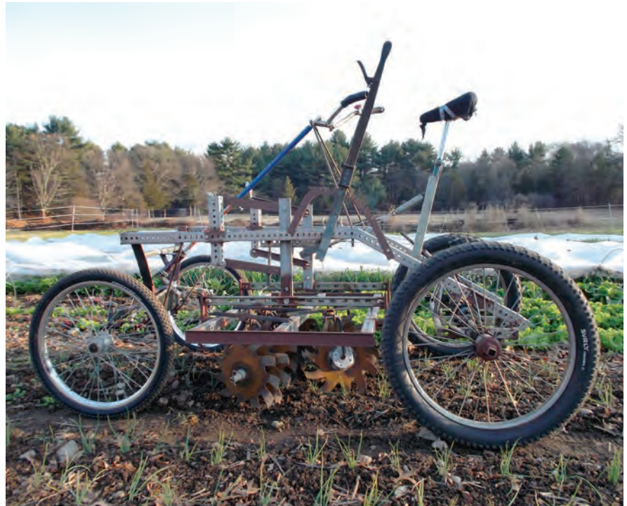
The Culticycle, an open-source pedal powered tractor for cultivation and seeding, built from readily available lawn tractor, ATV, and bicycle parts. Photo: Farm Hack
