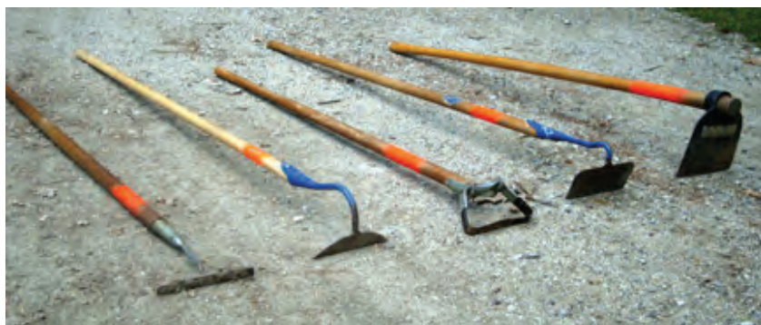
From left to right, a collinear hoe, a swan-neck hoe, a stirrup hoe, a "regular" hoe, and an eye-hoe. Photo: Andy Pressman, NCAT
