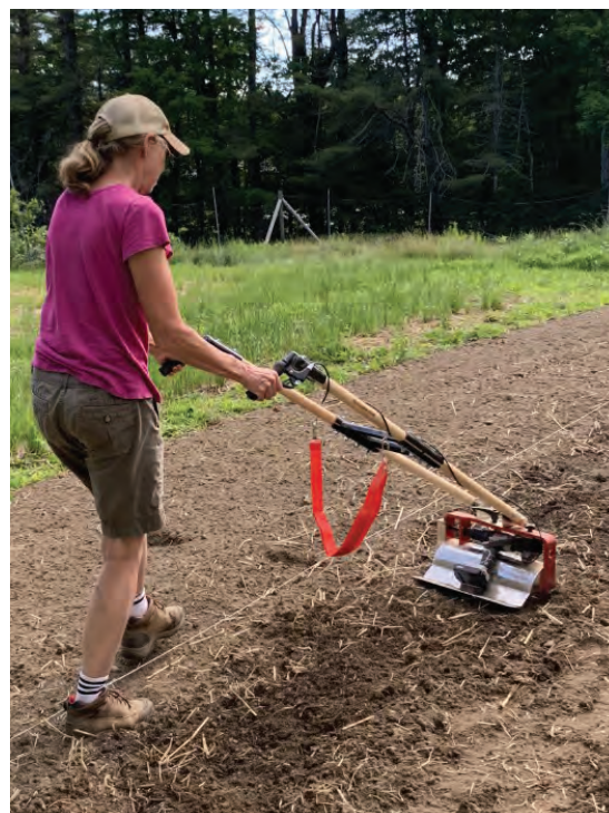
Drill-powered Iconoclast tool available from Neversink Farm. Photo: Andy Pressman, NCAT
