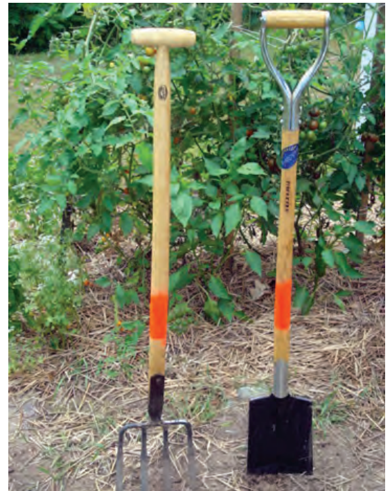
A digging fork (left) with a T-handle and a spade with a D-handle. Photo: Andy Pressman, NCAT
