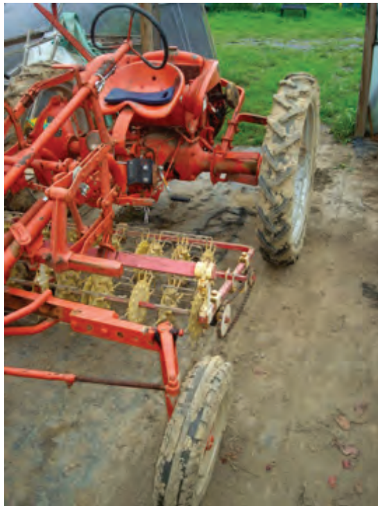
A basket weeder belly mounted to an Allis Chalmers G at Pennypack Farm and Education Center in Horsham, Pennsylvania. Photo: Andy Pressman, NCAT
