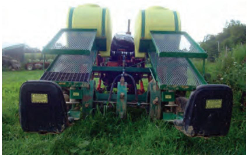
A Rainflo water-wheel transplanter at Pennypack Farm and Education Center in Horsham, Pennsylvania. Photo: Andy Pressman, NCAT
