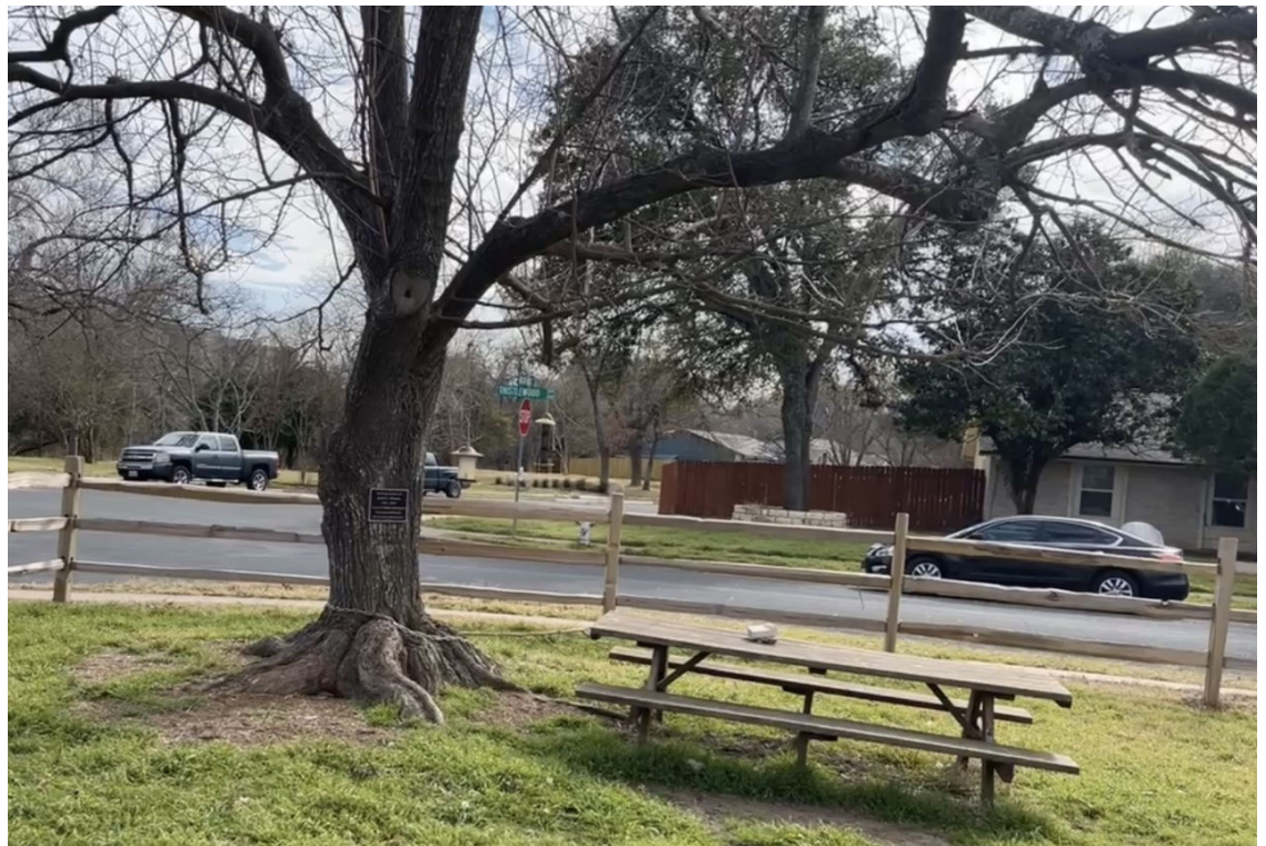
A floodplain-compliant table chained to a tree so it will not flow downstream in the event of a flood. Floodplain-compliant fencing is open, so that water is able to flow through. Photo: Katherine Favor, NCAT
