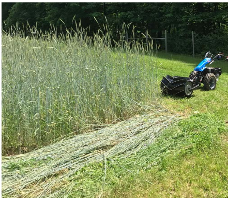
Top left: Walk-behind tractor with flail mower attachment. Photo: Andy Pressman, NCAT
