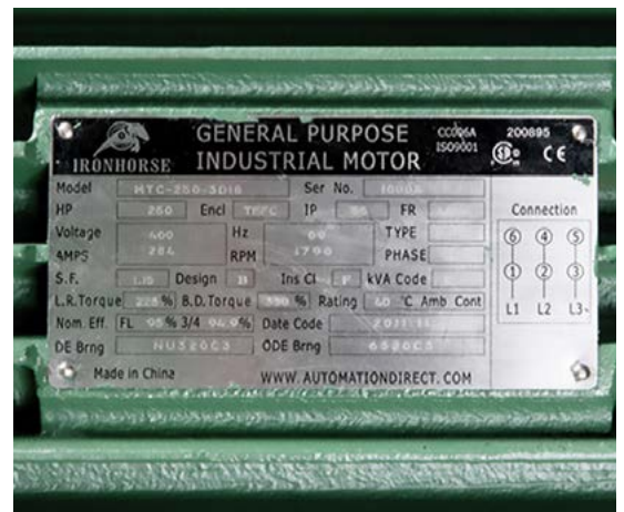
Figure 4. Nameplate of a 250-horsepower motor. Photo: NCAT
