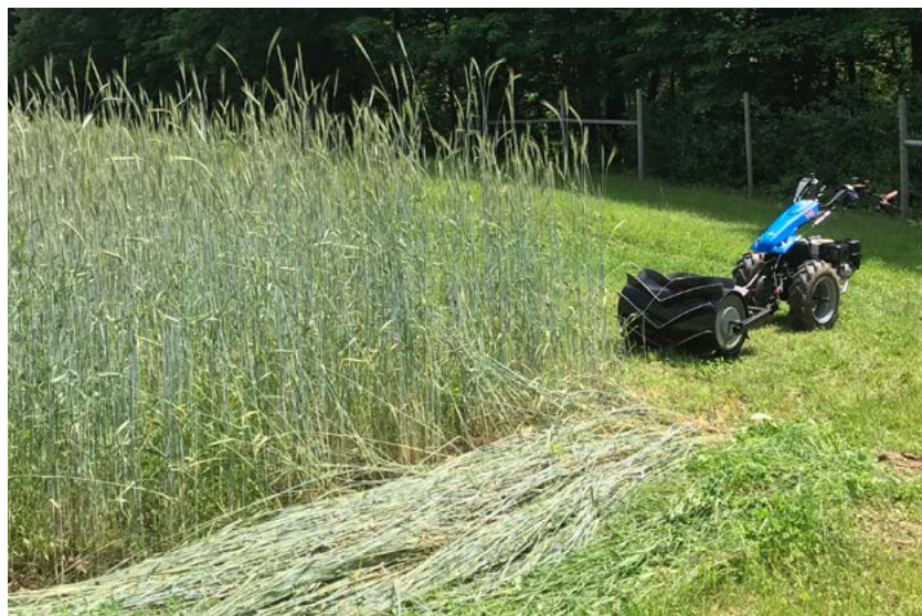
Rolling-crimping rye cover crop with a walk-behind tractor using roller-crimper attachment. Photo: Andy Pressman, NCAT
